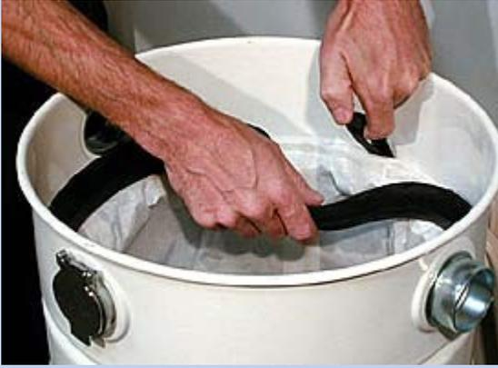
2. Remove the rubber gasket that is around the top of the filter bag by pulling gently on the edge of the rubber gasket. Remove from the canister.
