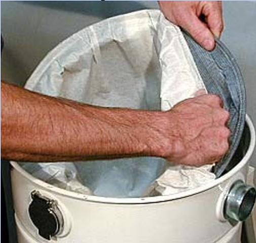
4. Remove the paper filter bag from the cloth bag by pulling the elastic edge of the paper filter bag upward from around the top metal ring of the cloth bag. Discard the paper filter bag.
